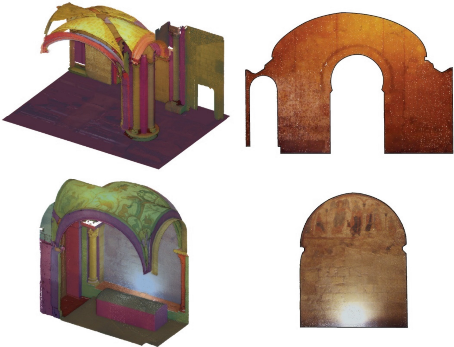
Fig. 2. Results of the RANSAC shape detection algorithm applied to the San Isidoro complex: The selected areas have been processed to extract the architectural elements.
