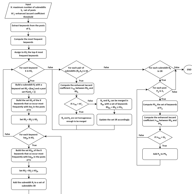
Fig. 10.2: A flowchart representing our approach to build virtual subreddits with homogeneous topics
