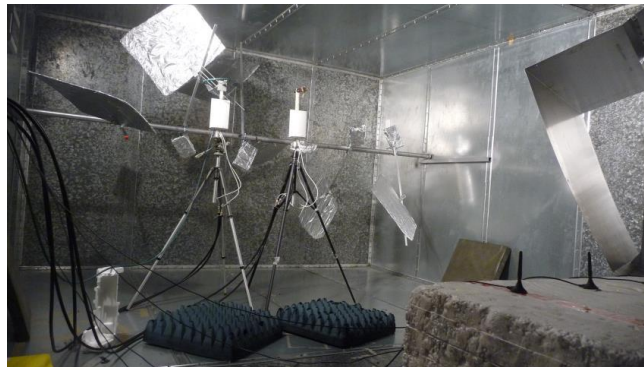
Figure 5: A typical outdoor antenna element for the 800 MHz and 1800 MHz LTE band brings a base station signal inside the RC. It is located a distance r from the UE (a dongle connected to a notebook), and some absorbing pyramidal and planar absorbers are put inside the RC.
