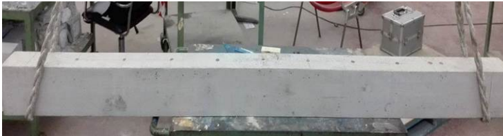
Figure 23 – (a) Set up of vibration tests on undamaged RC beams with hinge-hinge condition and instrumentation for dynamic tests; (b) beam hung to elastic springs and (c) accelerometer.
