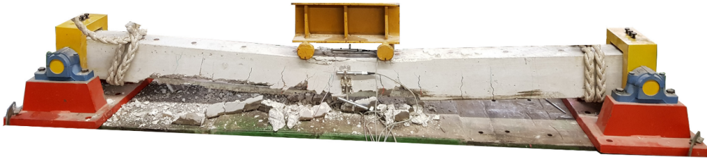
Figure 22 – Collapse view of strengthened beam B3 ( P \cong 33 kN).
