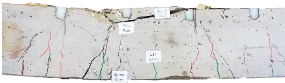
Figure 17 – View of failure of strengthened beam B2.
