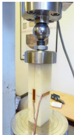
Figure 2 – Compression test of prismatic specimen of adhesive material.
