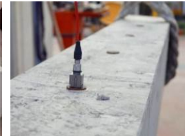
Figure 23 – (a) Set up of vibration tests on undamaged RC beams with hinge-hinge condition and instrumentation for dynamic tests; (b) beam hung to elastic springs and (c) accelerometer.
