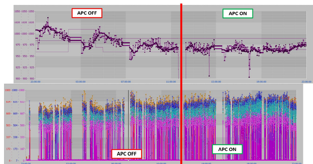
Figure 14. Control results: pre/post-APC system comparison (billets temperature at the rolling mill and rolling mill stands current absorptions).
