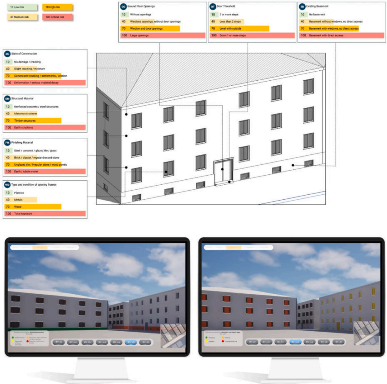
Fig. 7. VR mapping of construction elements based on BV attributes and descriptors (top) and output of false colour visualization of BV_eb (bottom left) and BV_wd (bottom right).
