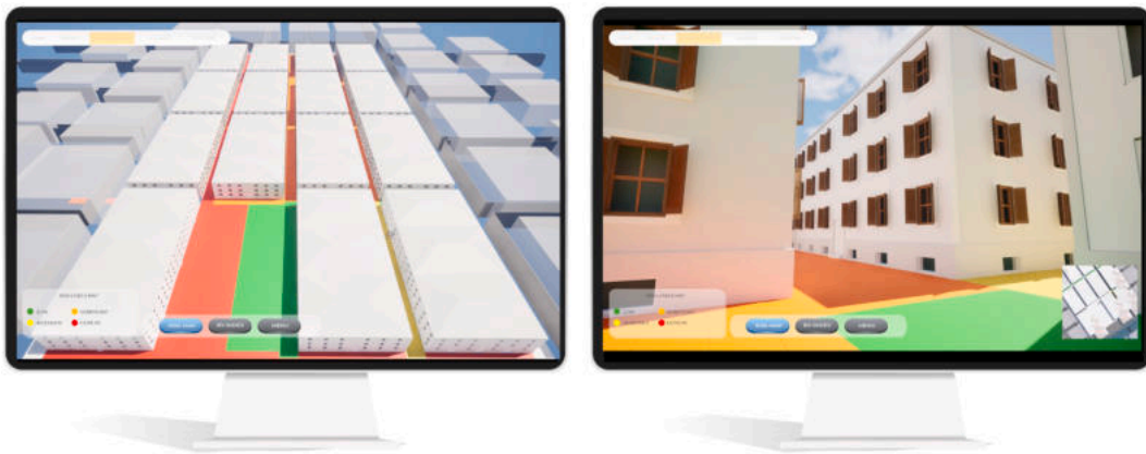
Fig. 9. VR mapping of open spaces according and hazard index D^*V : top-down (left) and ground-level views (right).
