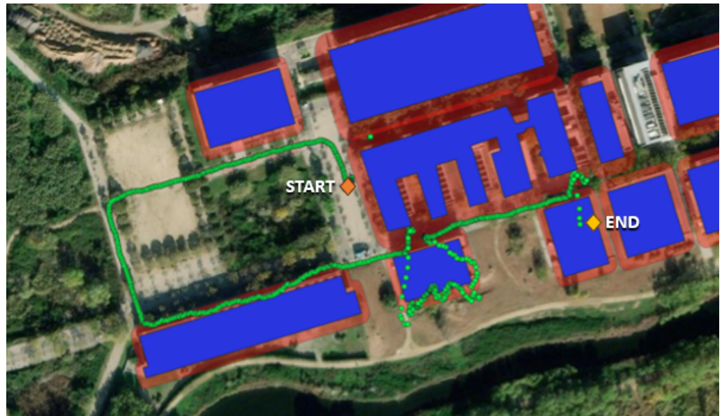
Figure 8. Transition or semi-outdoor area for the “PMT-LAB” (red) and GNSS-based trajectory (green). Building layouts are shown in blue.
