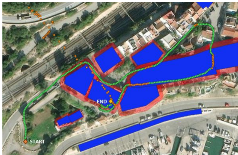
Figure 16. MK test applied to the trajectory in Garraf town. Green points are good GNSS areas, orange points are transitional areas from outdoor to indoor. Building layouts are shown in blue while transition or semi-outdoor area for the Garraf town is shown in red.
