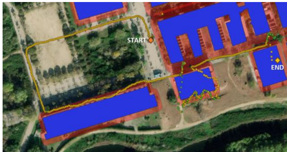
Figure 14. Slope test applied to the trajectory of “PMT-LAB”. Yellow points are points classified as good GNSS areas, while green points are points belonging to be transition or indoor areas. Building layouts are shown in blue, while transition or semi-outdoor area for the “PMT-LAB” is shown in red.
