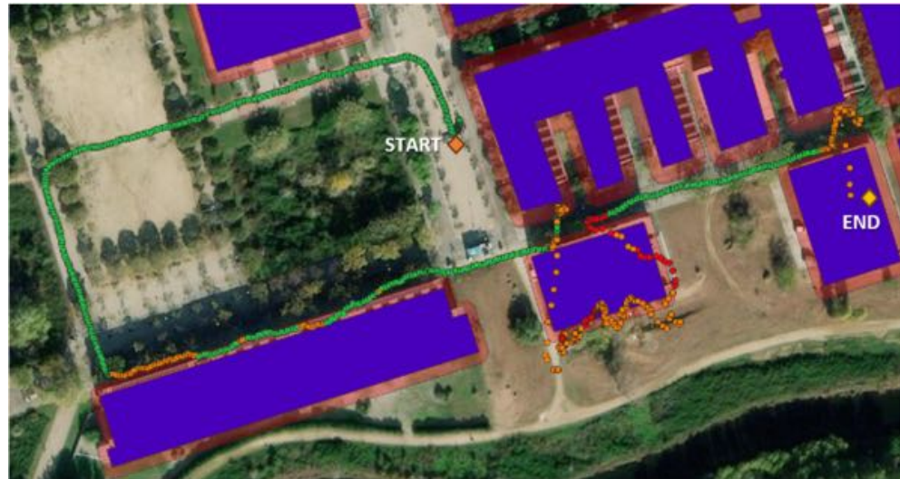
Figure 15. MK test applied to the trajectory of “PMT-LAB”. Green points are good GNSS areas, orange points are transitional areas from outdoor to indoor, and red are from indoor to outdoor. Building layouts are shown in blue, while transition or semi-outdoor area for the “PMT-LAB” is shown in red.
