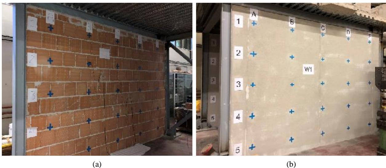
Figure 7. ILTs on infill masonry walls: (a) W2 before the plaster (P2), (b) W1 after the plaster (P3).
