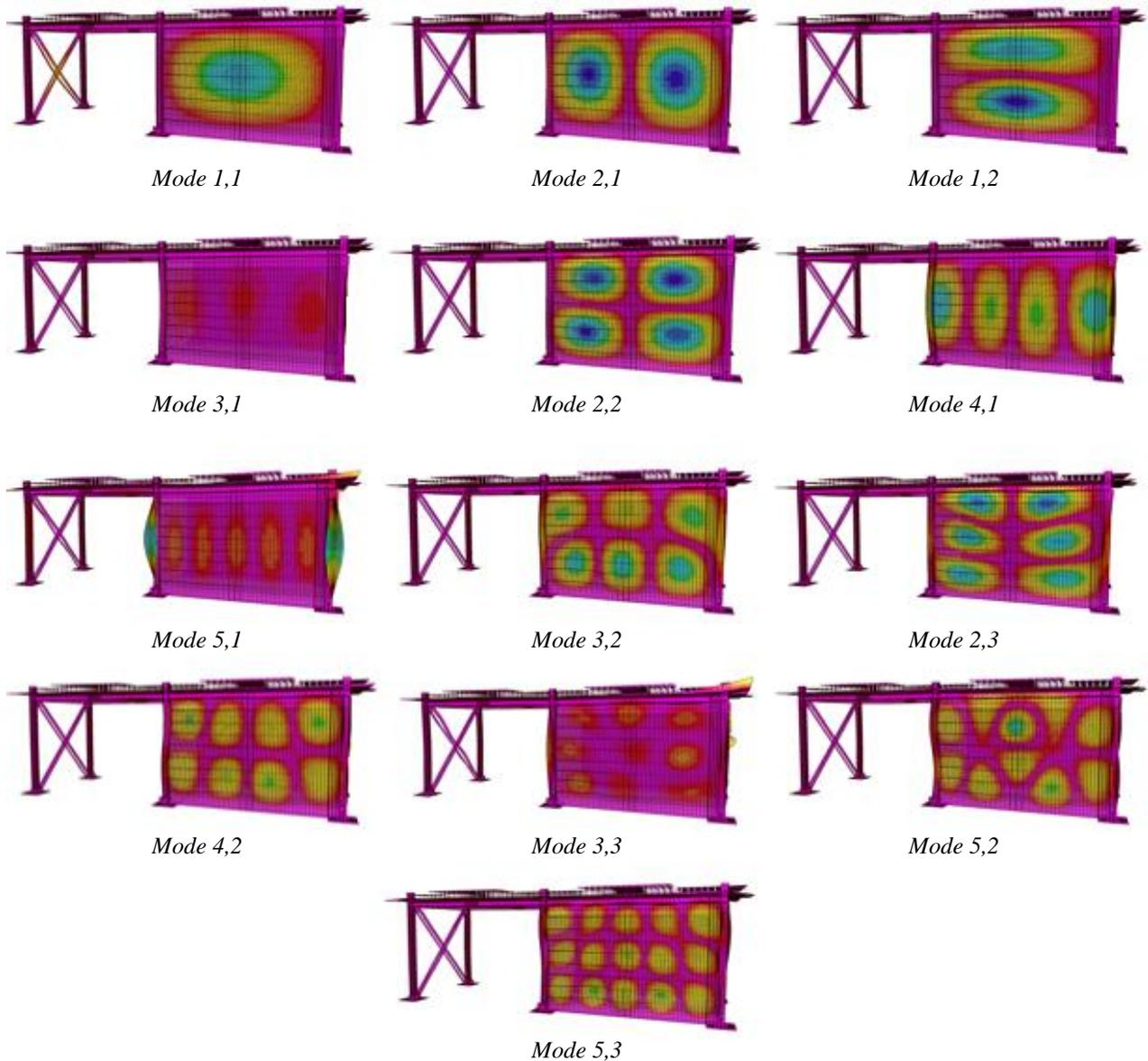
Figure 12. Infill numerical mode shapes within the global 3-D f.e. model.
