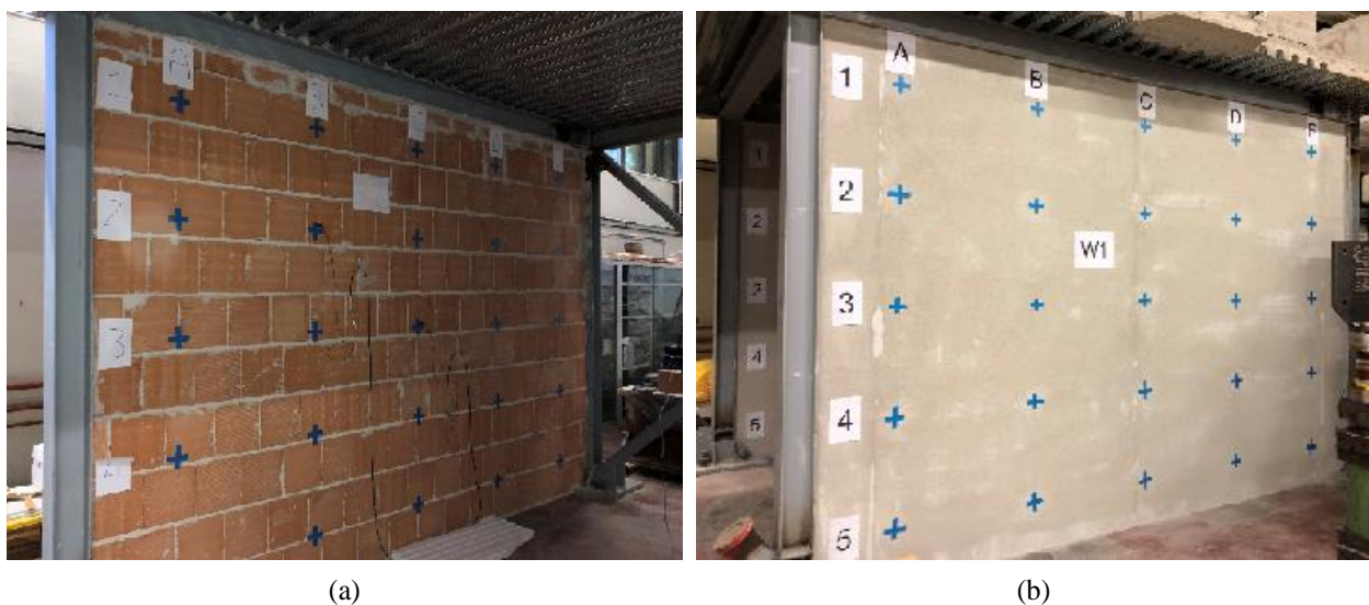
Figure 7. ILTs on infill masonry walls: (a) W2 before the plaster (P2), (b) W1 after the plaster (P3).
