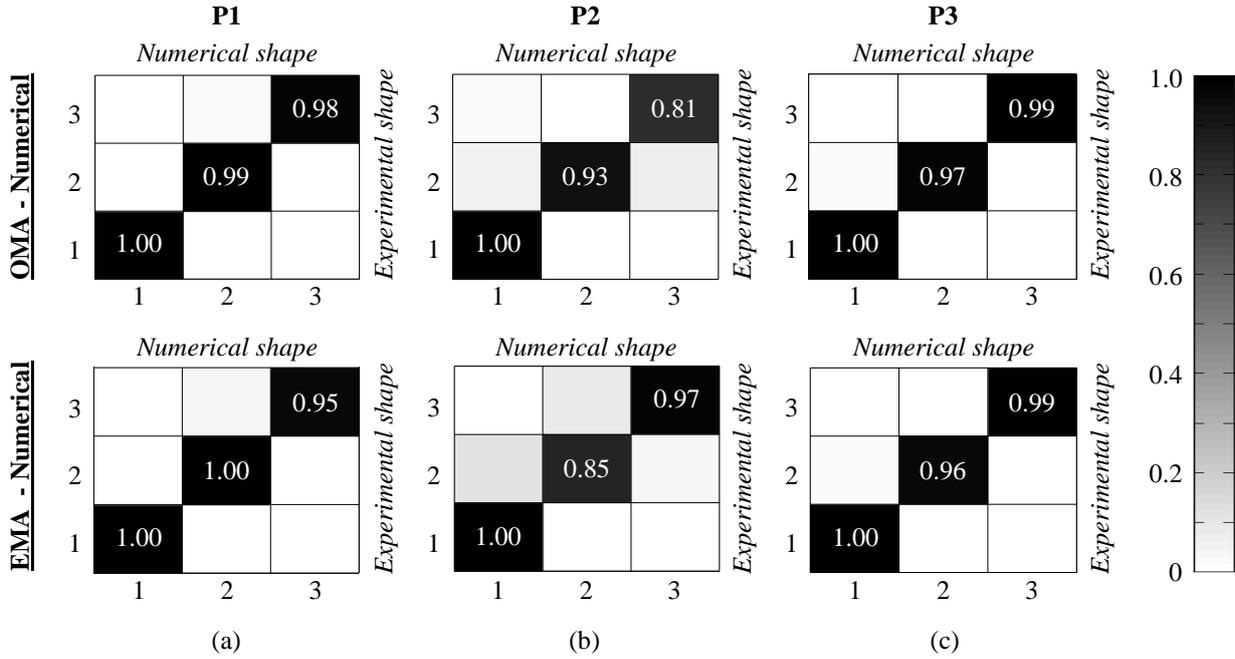
Figure 11. MAC indexes between experimental (OMA and EMA) and numerical mode shapes of the mock-up at different construction phases.
