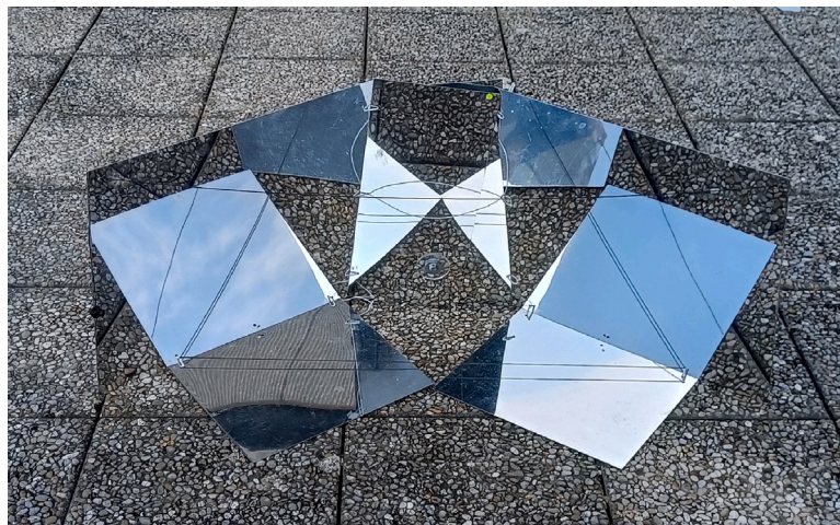
Fig. 4. Configuration of the Kimono for low sun elevation (lower than 40^\circ ).
