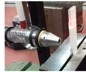
Fig. 7. Set-up for vibrational excitation by volume acoustic source
