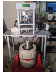
Fig. 6. Load system for DIC and TSA.
