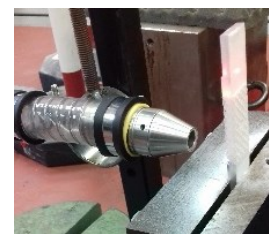
Fig. 7. Set-up for vibrational excitation by volume acoustic source
