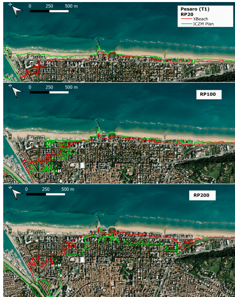
Fig. 10. Inundation perimeters for Pesaro (T1) and for different return periods (20, 100, 200 years). Red and green lines represent the perimeters computed by XBeach and that reported in the ICZM Plan. (For interpretation of the references to color in this figure legend, the reader is referred to the web version of this article.)
