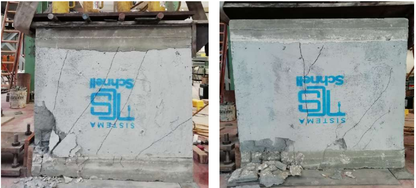
Figure 17. Shear test with constant compression: crack patterns at failure
