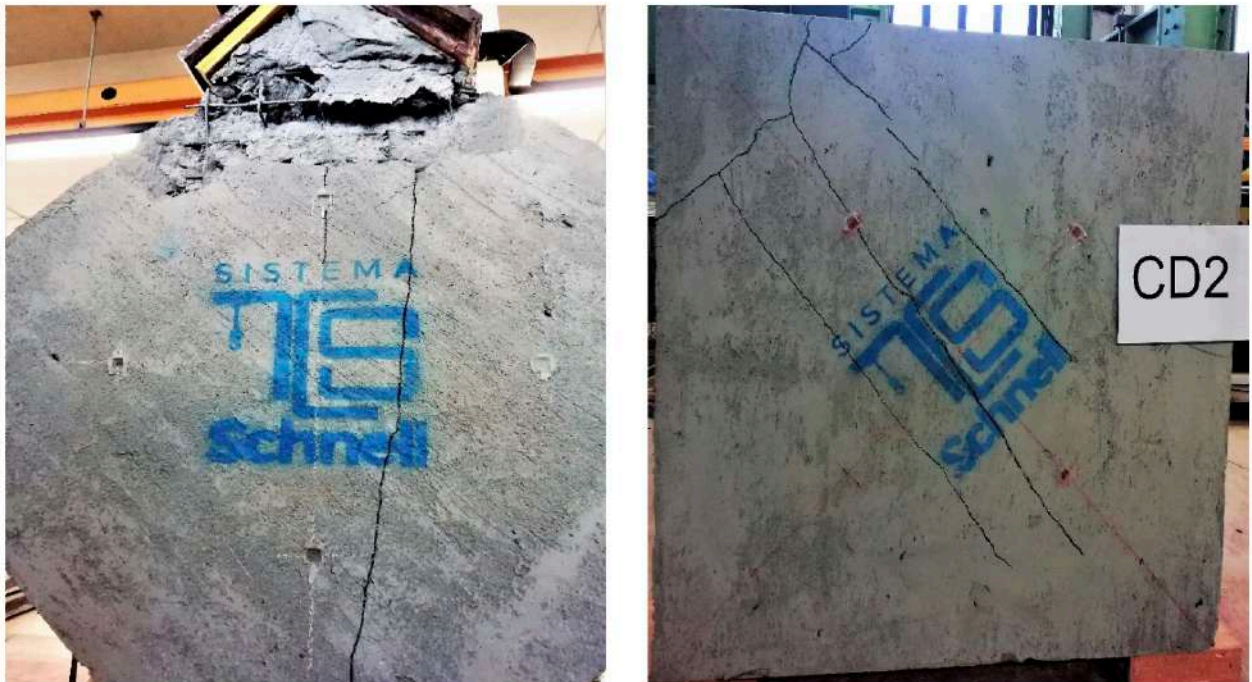
Figure 15. Diagonal compression test: crack patterns at failure
