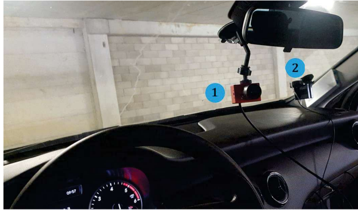
Figure 6.3: Detail of vision system, with the dashboard of the prototype car fitted with (1) the DVS camera and (2) the GNSS receiver.
