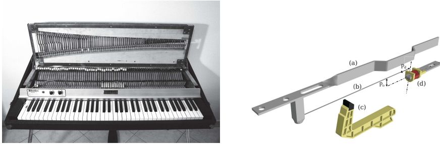
(a) Overall view of Mark I Stage Rhodes. (b) Details of the Rhodes F1 tuning fork.
