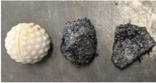
Fig. 3. Comparison between the spherical sensor and coarse aggregates from the DGBC mixture.
