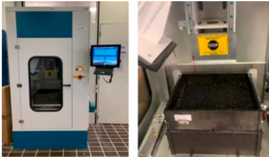
Fig. 7. Roller compactor by Infratest.
