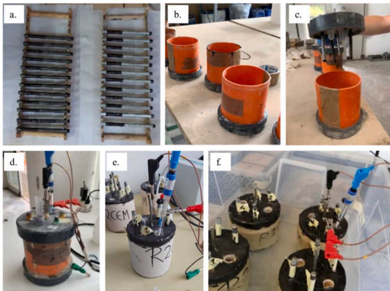
Fig. 1. Reinforced cylindrical specimens preparation: a. coated rebars, b. cylindrical molds, c. cylindrical mold with cover, d. corrosion measurements on specimens inside the molds, e. corrosion measurements on specimens outside the molds, f. corrosion measurements on specimens during wet/dry cycles in tap water (in the picture, measurements in wet condition are shown).
