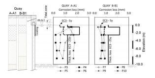
Figure 8. Corrosion loss evaluated from nominal thickness of the profiles compared with corrosion profiles suggested by Eurocode 3 for 25 y ( $\Box\Box\Box$ ) and 5 y (- - -) of exposure
