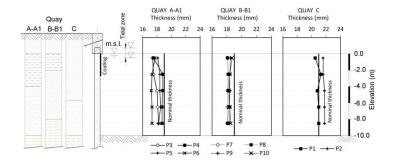
Figure 7. Measurements of the thickness of the steel profiles at different depth
