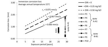
Figure 9. Measured corrosion losses compared with the linear model predictions according to Melchers and Jeffrey (2014)
