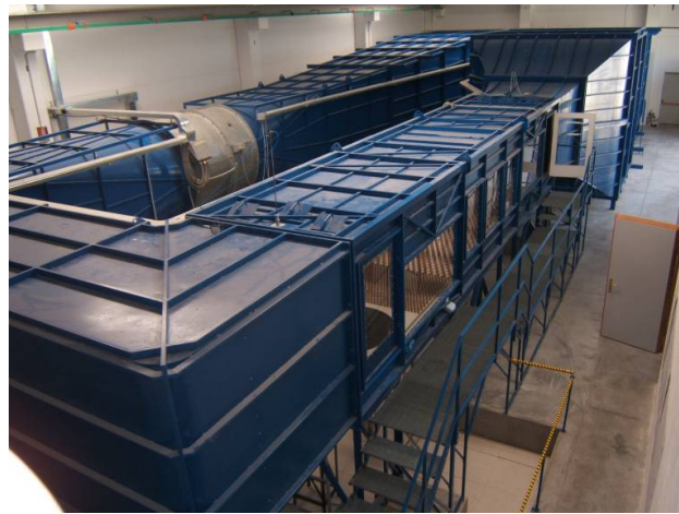
Fig. 3: The Environmental Wind Tunnel of the Marche Polytechnic University
