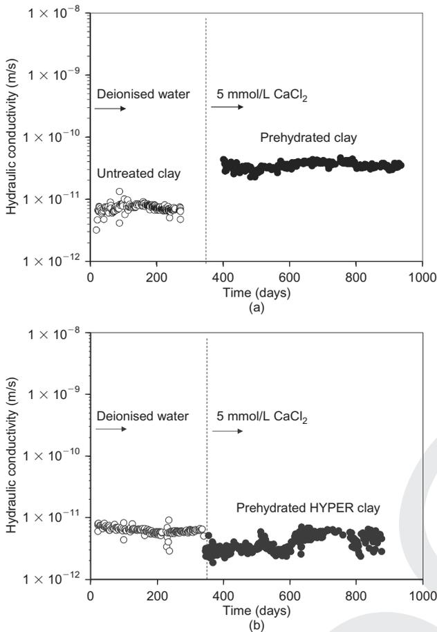
**Figure 5.** Hydraulic conductivity to 5 mmol/L CaCl<sub>2</sub> solution of: (a) untreated clay and (b) the HYPER clay after prehydration with water
