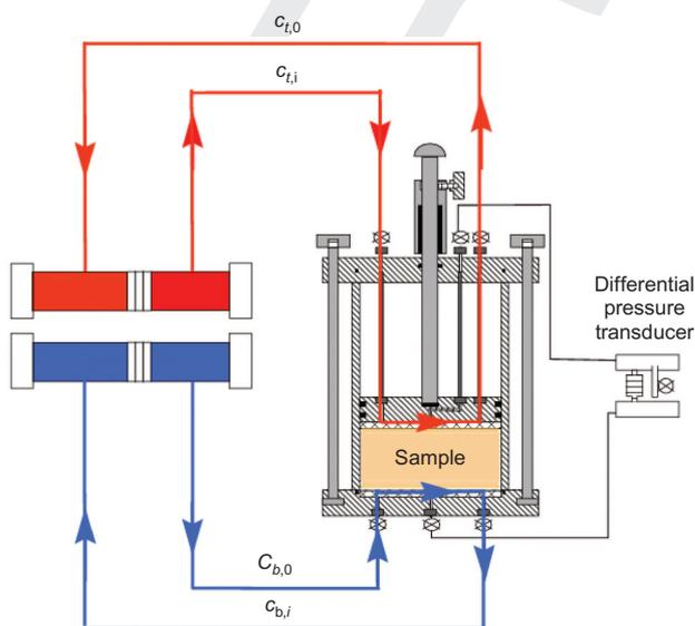
**Figure 1. Chemico-osmotic test experimental setup**
