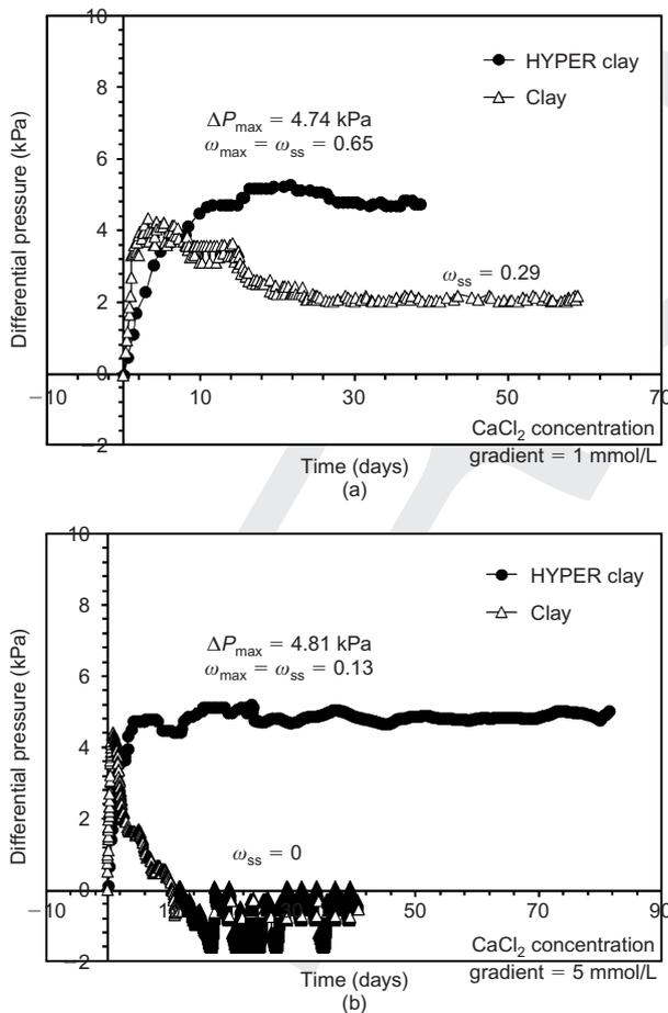
Figure 8. Enhancement due to the anionic polymer (CMC) on the chemico-osmotic efficiency of the HYPER clay with a concentration gradient: (a)  $\Delta C_1 = 1 \text{ mmol/L CaCl}_2$  and (b)  $\Delta C_2 = 5 \text{ mmol/L CaCl}_2$
