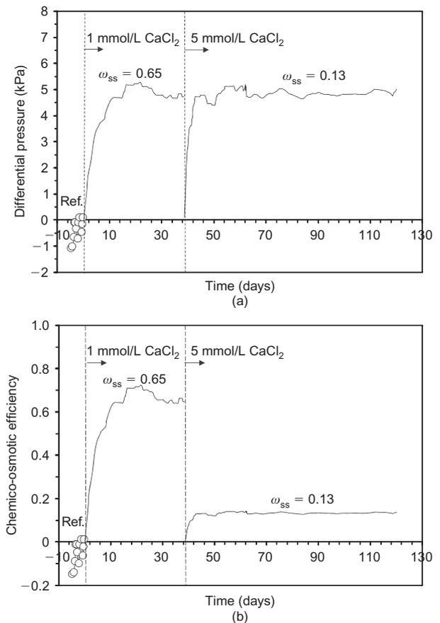
**Figure 7. (a) Chemico-osmotic induced differential pressures and (b) chemico-osmotic efficiency of the HYPER clay for multiple-stage test (concentration gradients  $\Delta C_1 = 1$  mmol/L CaCl<sub>2</sub> and  $\Delta C_2 = 5$  mmol/L CaCl<sub>2</sub>)**
