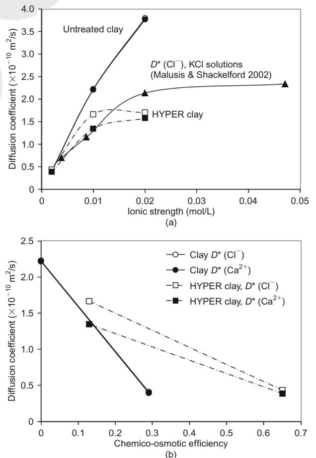
Figure 9. Effective solute diffusion coefficients plotted against: (a) ionic strength and (b) chemico-osmotic efficiency (data of HYPER clay with  $10 \text{ mmol/L CaCl}_2$ , ionic strength  $0.02 \text{ mmol/L}$ , from Seurynek 2012)
