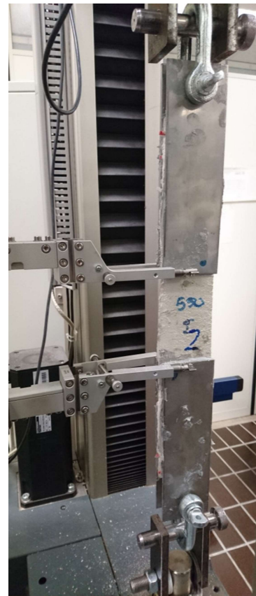
Fig. 4 – FRCM tensile test setup: strains measured with macro extensometer
