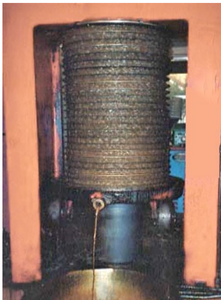
Figure 32: Extraction by pressure with presses (by website https://www.elicriso.it/it/olio/estrazione_olio_olive/ )
