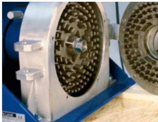
Figure 28: Toothed disc crusher (P. Amirante et al., 2010)
