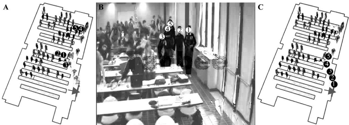
Fig. 11. A plan of the evacuation phase for the students leaving first (numbered people): on the left, the students' initial positions at the sounding of the fire alarm (A), in the middle, a frame of the experimental evacuation videotape, about 22 s from the sounding of
