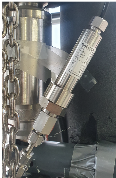
(a) Reference sensor Keller PA-33X mounted on the rig.
