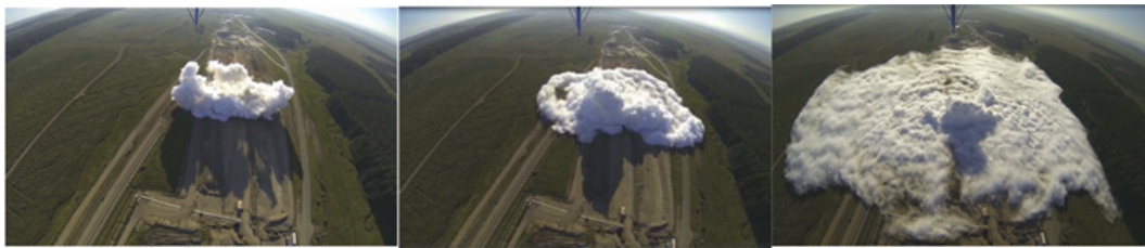
Figure 3.10.: The visible cloud behavior after the rupture; from left to right, at 10, 30 and 120 s from the break (From Ahmad et al. [10], Copyright Elsevier, 2015).
