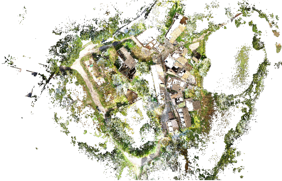
Figure 3.23: Point cloud obtained from the terrestrial LIDAR survey (top view).
