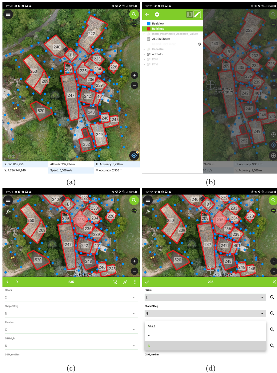
Figure 4.10: Screenshots of the QField application with the data generated inside the QGIS project: (a) General view of the cadastral layer, the ortophoto and the point layer that represents the different scan stations; (b) View of the project tree; (c) Appearance of the app when the user consults the data contained in a shapefile and (d) Appearance of the app when the user edits a field.
