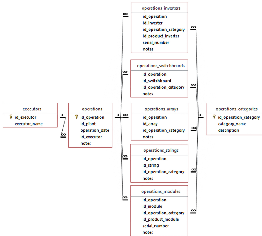
Figure 3.10: The operations group of the conceptual model implemented into the relational database.
