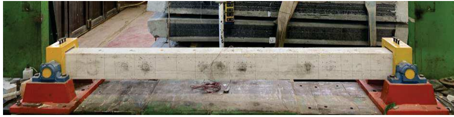
Figure 5.7 – Set up of vibration tests with hinged ends
