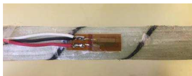
Figure 4.2 – Strain gauges on FRP bar
