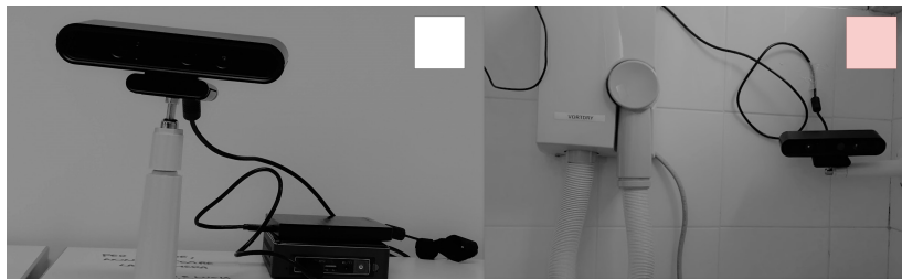
Figure 3.1: The acquisition set-up (white square, left), placed in the bathroom to record the sink (pink square, right), consisted of an Astra Mini S-Orbbec® RGB-D camera and a minipc Intel® NUC core i5.
