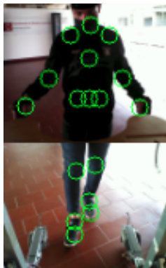
Figure 4.6: Chosen percentage of correct keypoints ( PCK ) threshold radius of 6 pixels. Detection values inside the circles, for each keypoint, are considered correctly detected.
