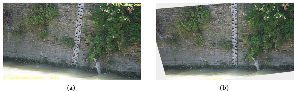
Figure 7. Image ortho-rectification example. (a) The original frame sent by the V-IoT device; (b) The frame after ortho-rectification based on specific site's setting.
