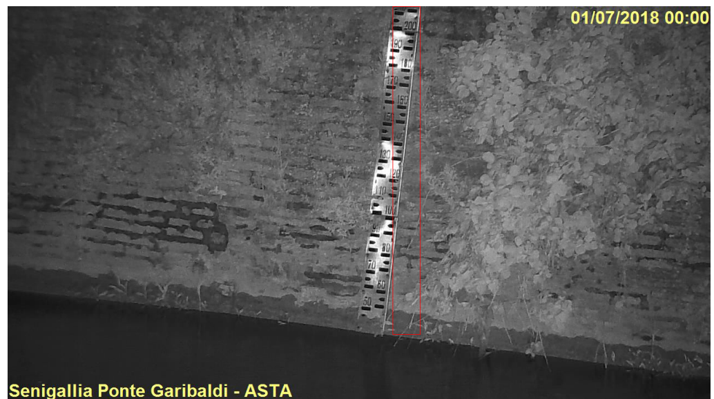
Figure 6. The original frame with the desired gauge positioning, used to compute image rectification settings.
