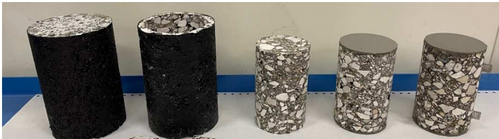
Figure 57 - Preparation of the specimen for the dynamic modulus test
