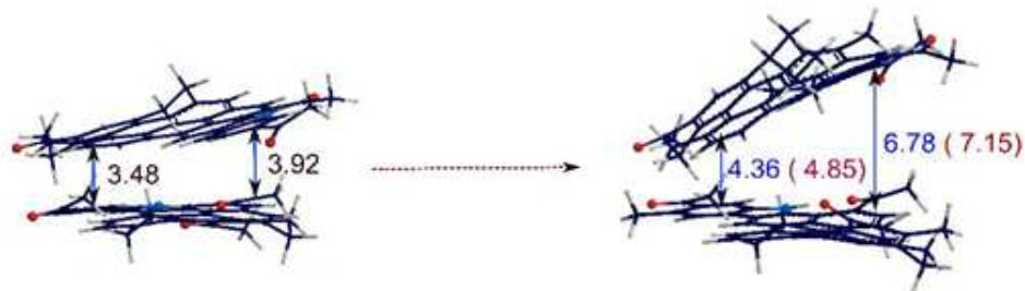
Figure 12 - Intermolecular gaps between the aromatic rings in zones A-B and C for an oxidized dimer before (left) and after (right) rejuvenation. Blue and red numbers indicate the distances (in Å) achieved with 2 different rejuvenators (Reprinted with permission)
