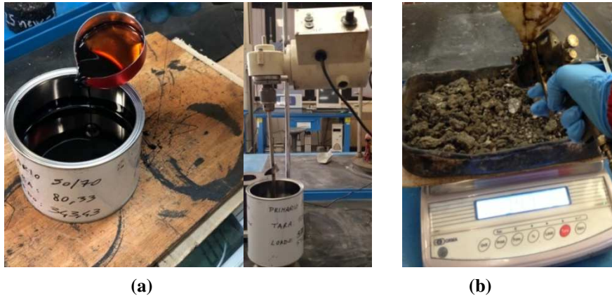
Figure 40 - addition and mixing of additives A, C, D, E, F, G in the virgin bitumen (a) - addition of rejuvenator B sprayed directly on the RAP (B)
