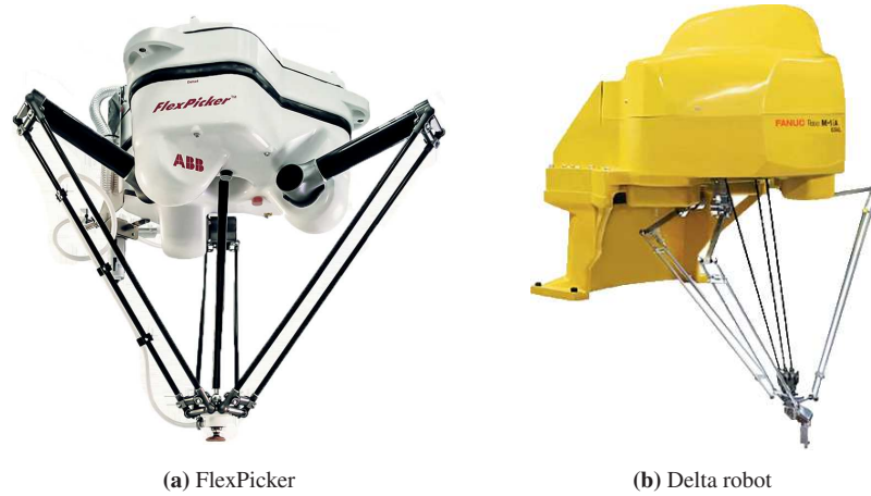
Figure 1.1.: Industrial robots with slender links. Courtesy of ABB (left) and Fanuc (right)
