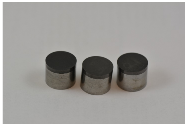
Figure 14. Inserts for drill tools drill tools, which consist of a polycrystalline diamond layer (black colour) on a cemented carbide substrate, inserts diameter is 12.5 mm.
