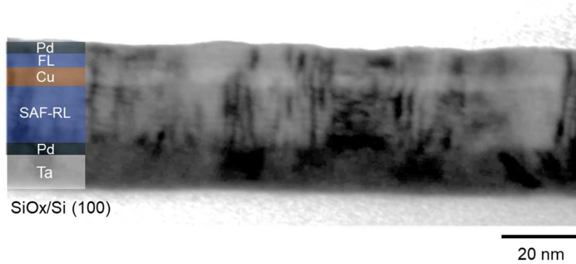
Figure 3.6. Cross section TEM bright-field image of a GMR-SV thin film stack ( t_{Cu} = 3 nm) on SiO 2 /Si (100).
