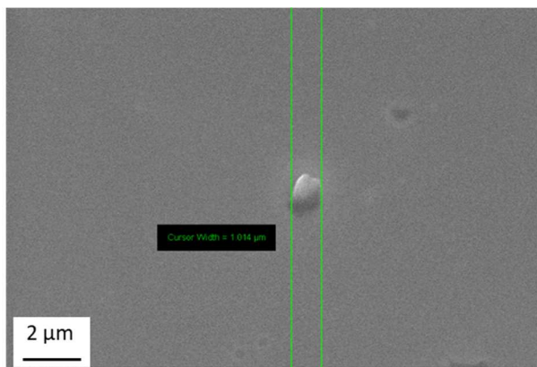
Figure 5.11. SEM image of the microdisks obtained after dissolving the sacrificial resist.
