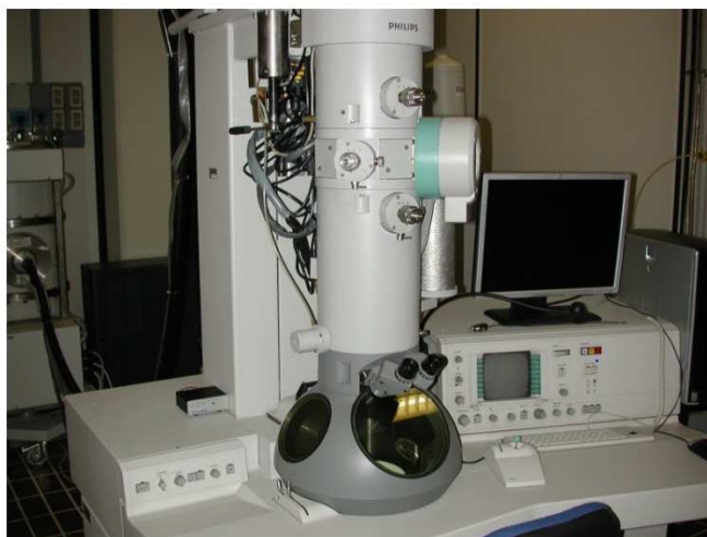
Figure 2.12. A Philips CM200 microscope used for TEM characterization during this PhD thesis.
