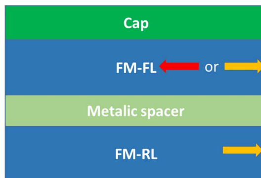
Figure 1.5. Illustrative sketch of a spin valve structure with in-plane magnetic anisotropy, FL and RL stand for the free and reference layers respectively.
