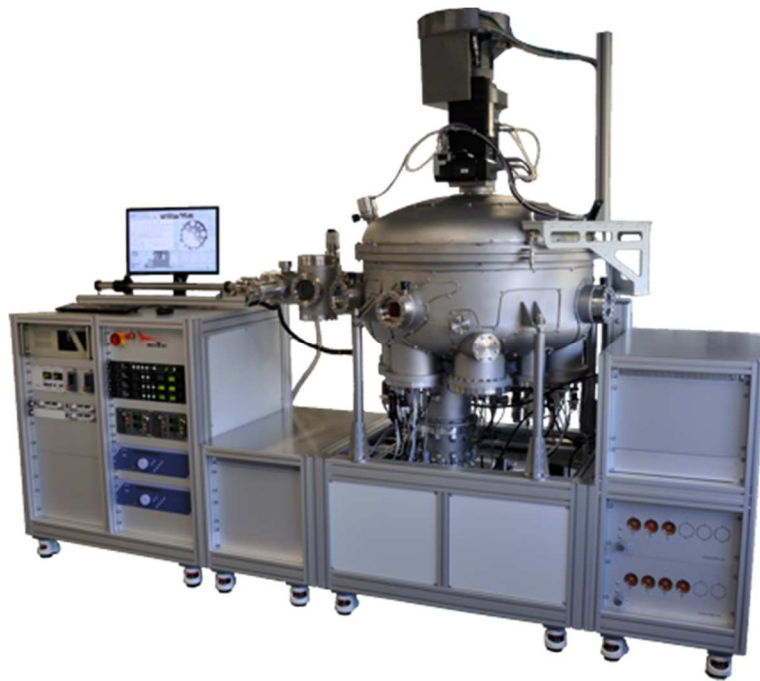
Figure 2.3. UHV sputter deposition system
