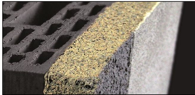
Figure 3.3.1 Hydraulic lime-based plaster realized with natural organic aggregates (cork) for thermal insulation and acoustic absorption
