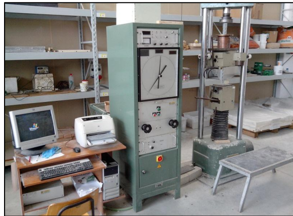
Figure 3.5.3" Galdabini" Hydraulic press for mechanical tests
