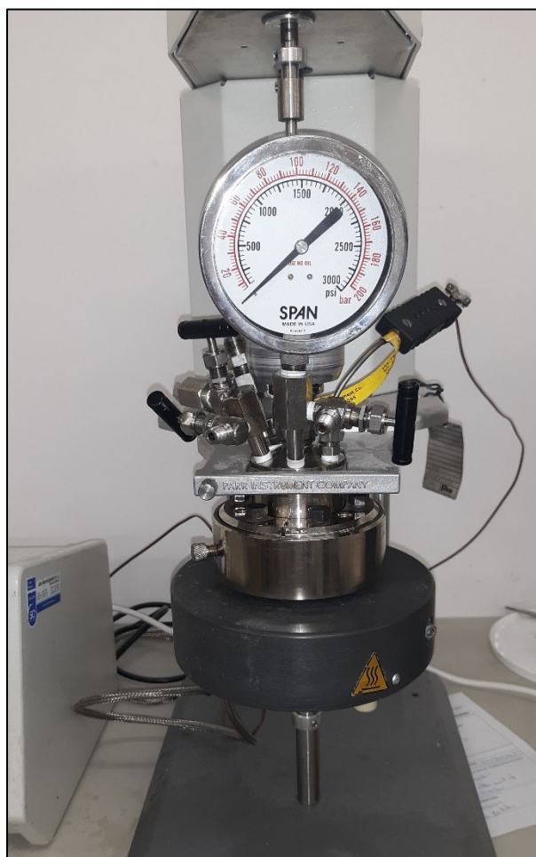
Figure 7.5.3 Parr Reactor (100 mL capacity)
