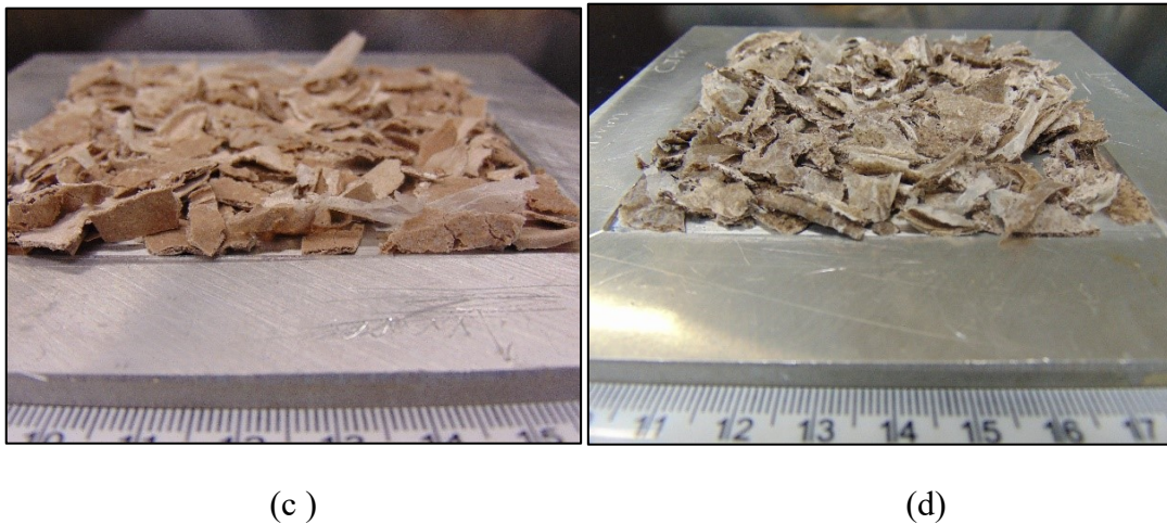
Figure 6.6.1 Preparation of the cut film in the mould for the compression moulding process: a) 100% PHA (CP_Pm); b) 70%PHA +30% WF (CP_30WF_Pm); c) 70%PHA +30% MS (CP_30MS_Pm);d) 70%PHA +30% CG (CP_30CG_Pm).
