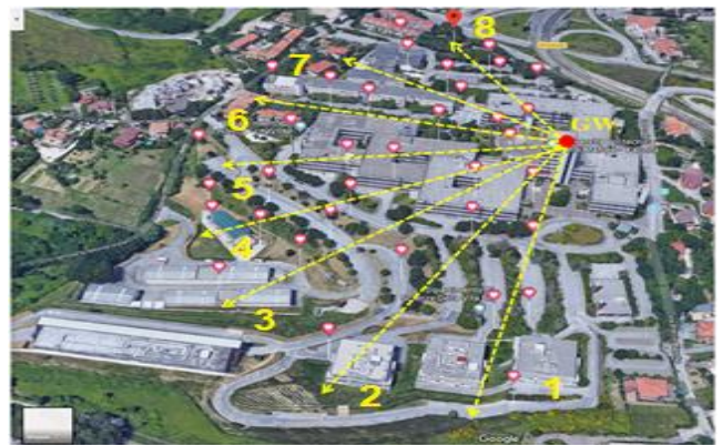
Figure 2. The 37 planned LoRa RSSI measurement positions along eight different directions within the university campus.
