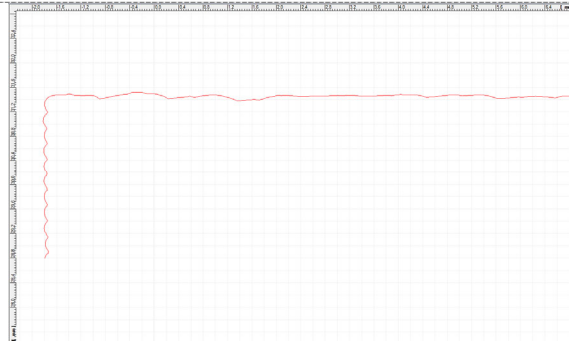
Figure 7. Profile shape of specimen B in the Z direction and on the top surface.
