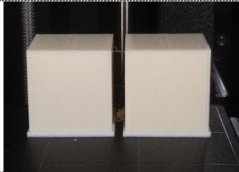
Figure 2. Specimens realized with Fused Deposition Modeling.
