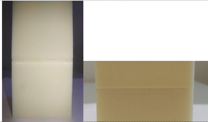
Figure 9. Assembly problems at macro-contact level of the built specimens.
