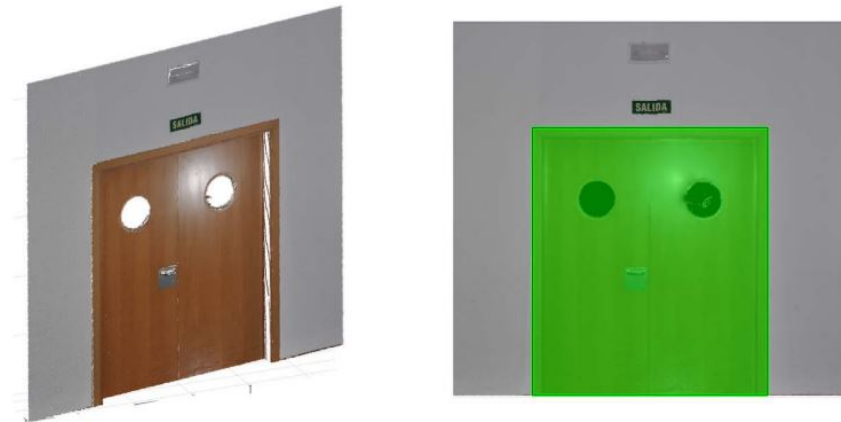
Figure 2.12: Detection results for Simple Scenes. (Left) Original 4D orthoimages. (Right) Door detection [Quintana et al., 2018].
