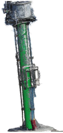
Figure 2.7: Primitive modeling of a cylinder indicating a piece of a pipe [Rodriguez-gonzalvez et al., 2014]
