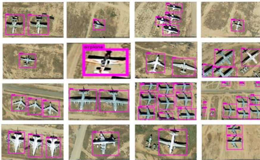
Figure 2.18: Airplane aerial images for object detection with YOLO [Radovic et al., 2017].
