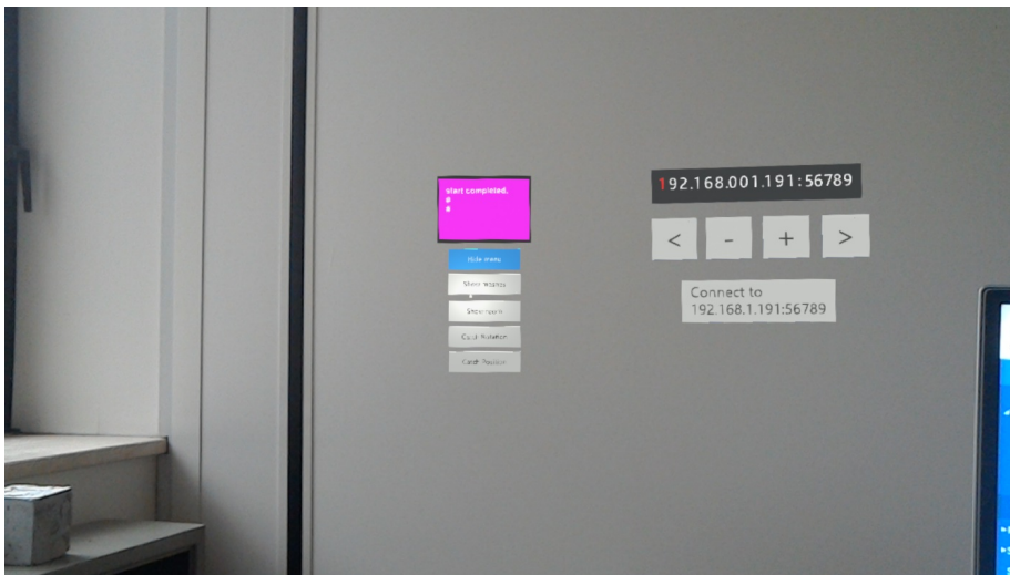
Figure 5.11: Application interface for HoloLens connection to embedded system.
