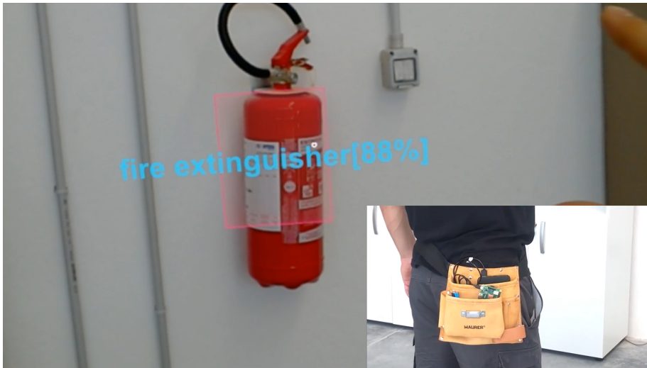
Figure 3.29: Real-world validation of the customized network for fire extinguisher recognition.
