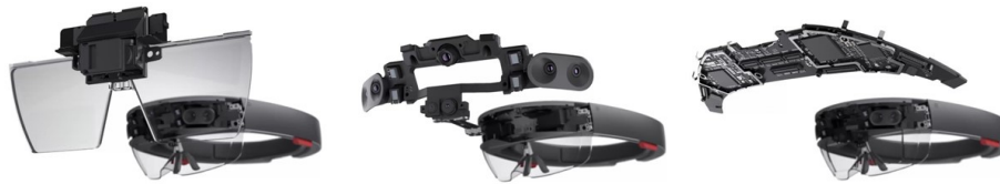
Figure 3.34: HoloLens display, sensor and processor [Microsoft, 2018c].
