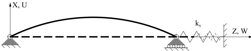
Figure 2.3: Configuration of the beam-spring system.
