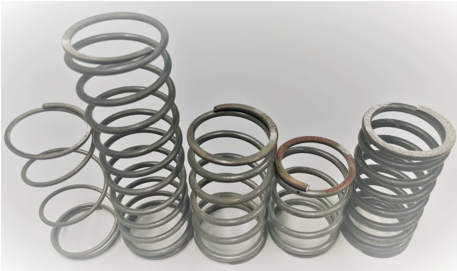
Figure 4.2: Springs from the least to the most stiff (from left to right): 67 \times 28.5 \times 1.8 mm, 100 \times 32.5 \times 2.5 mm, 60 \times 35 \times 3 mm, 43.5 \times 33.5 \times 3 mm, 61 \times 33.5 \times 3.5 mm.
