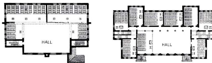
Fig. 1-4 (1) School in Paisley (England). First half of the nineteenth century. The hall can be joined to the classrooms by opening sliding walls. Source: Carbonara P. [1958], Gli edifici per l'istruzione e la cultura , p.845. (2) School in Johnson Street, London (England). Second half of the nineteenth century. The hall is separated from the classrooms. Source: Carbonara P. [1958], Gli edifici per l'istruzione e la cultura , p.845.
