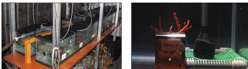
Figure 1. Experimental apparatus used for simulating particle resuspension.
