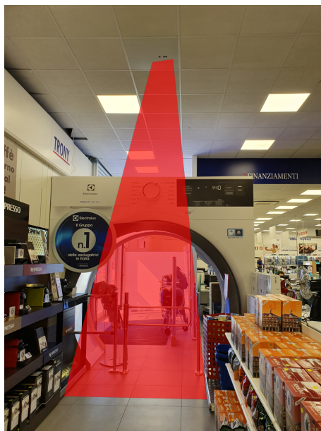
Figure 1.2: Typical entrance camera installation for people counting and re-identification.
