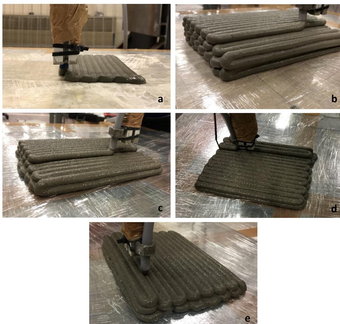
Figura 9.5 – Estrusione delle lastre: (a) RIF; (b) SAND50-PWD50; (c) PWD100; (d) PWD50-GRAN50; (e) PWD25-GRAN75
