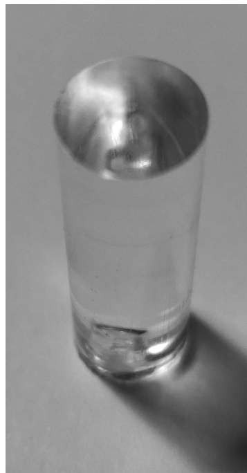
Figure 4.13: Quality control system for burrs identification: Smooth end exit coupled with the second illuminator to transmit light.
