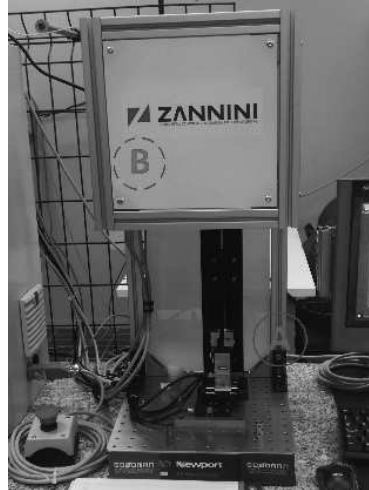
Figure 3.28: Confocal chromatic sensor quality control system for geometric feature assessment: change in the positioning of the temperature sensor.
