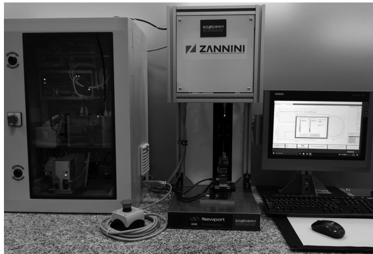
Figure 3.23: Confocal chromatic sensor quality control system for geometric feature assessment: laboratory measurement setup.
