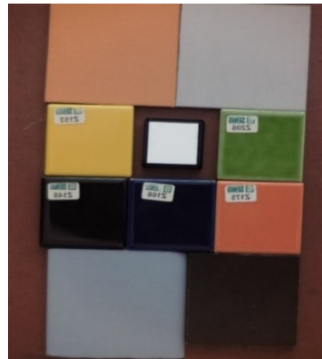
Figure 43 The 9 reference tiles used for the colour validation procedure and the whit target (D65 illuminant) in the centre.
