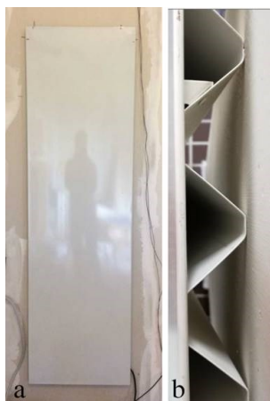
Figure 3.11: (a) Front view of the electric radiator and (b) top view of the tubular section.
