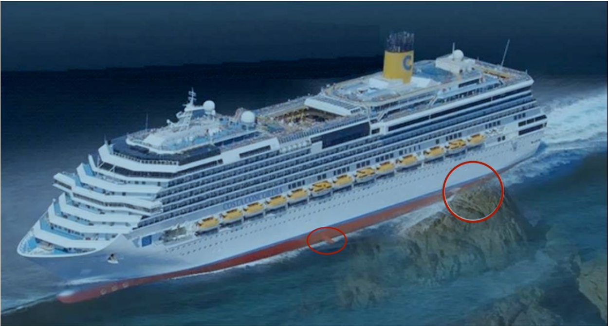
Figure 3 - Overview of the impact of the Costa Concordia with the Scioe rocks. the points where the ship collides with the rocks are highlighted by red circles (Source: final judgment in the first instance criminal proceedings against Francesco Schettino).
