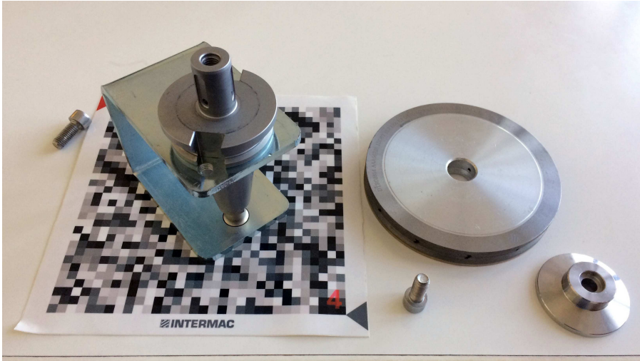
Figure 3.19: Example of a real component used for the development of this showcase; in particular, the object is a cone that one has to mount over a machine for glass moulding.
