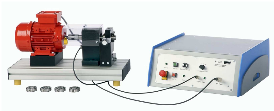
Figure 6.1: Bearing Faults Simulator.
