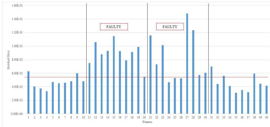
Figure 7.4: Example of residual error for 4 different sequences associated to 2 faulty motors and 2 normal motors.
