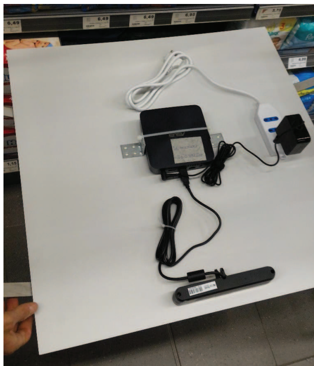
Figure 4.7: Configuration hardware of Shopper Analytics mounted on ceiling.
