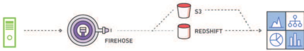
Figure 4.4: Data workflow implemented with Amazon AWS services.
