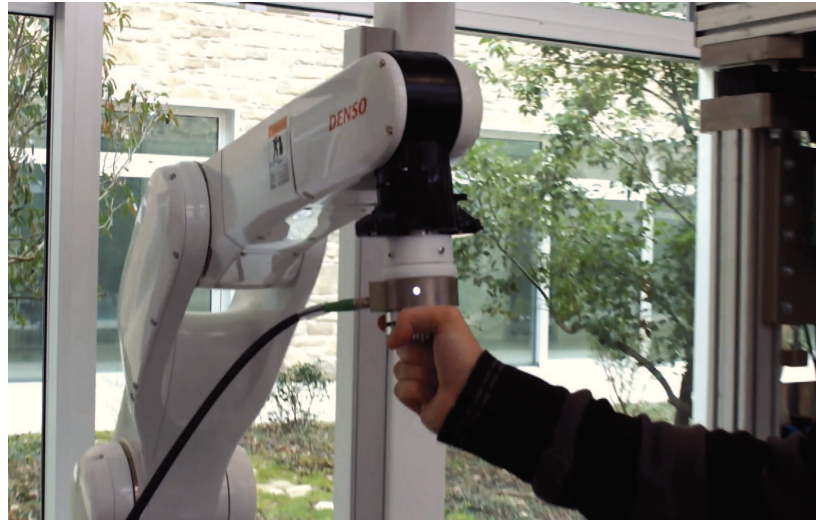
Figure 5.2: Denso industrial robot in manual guidance control.
