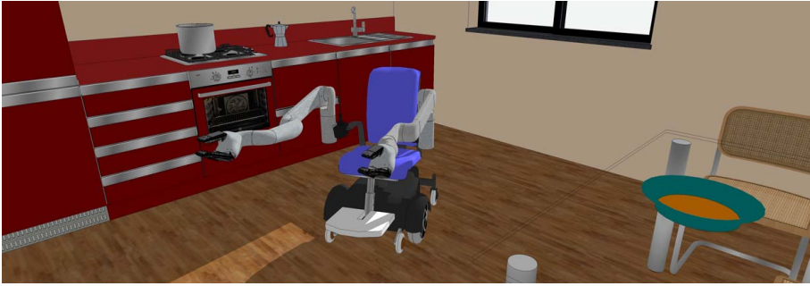
Figure 5.1: Concept of the wheelchair with two manipulators within an AAL scenario
