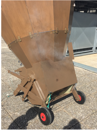
Figure 3.7: Smoke from the solar box cooker during an experimental test.
