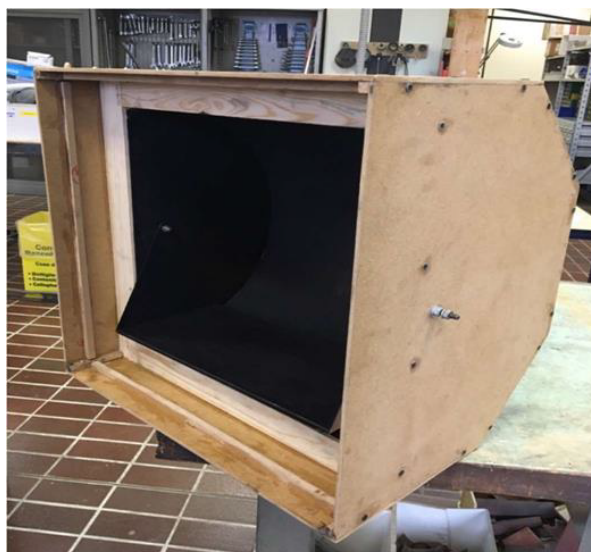
Figure 6.6: Cooking chamber built into the external wooden structure.
