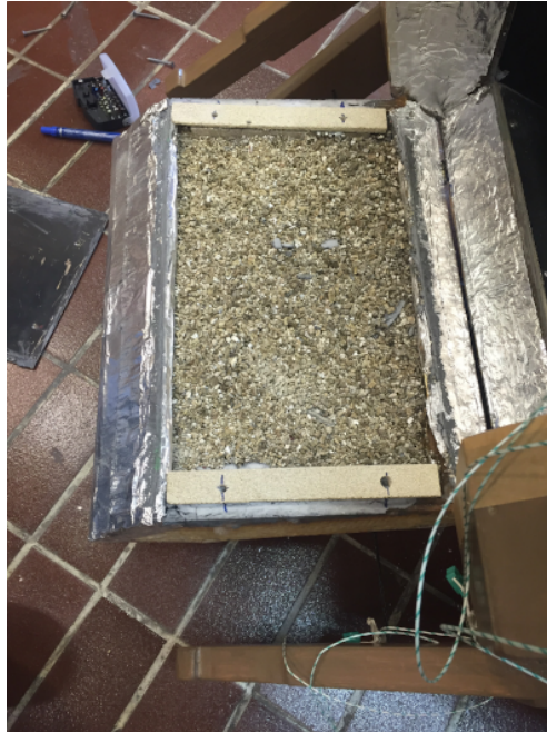
Figure 3.8: Vermiculite inserted in the small door cavity.
