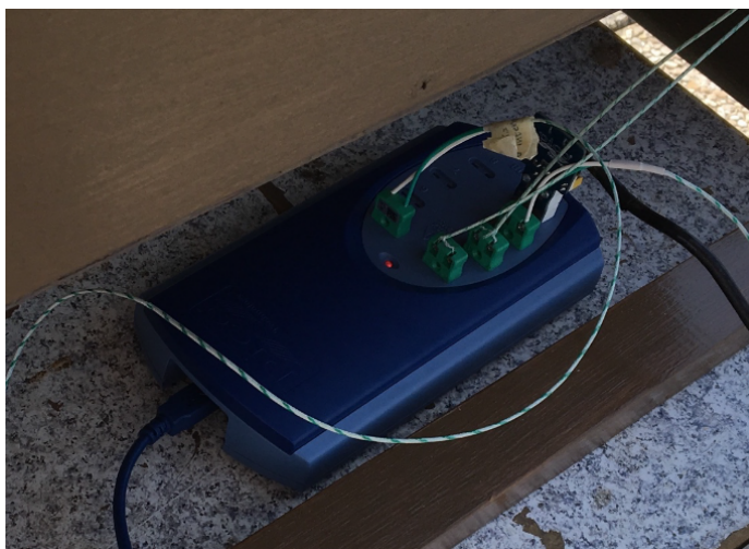
Figure B.2: Thermocouples linked to the acquisition system.
