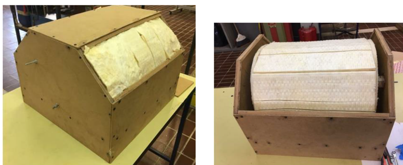
Figure 6.7: Glass wool layers and flakes inserted in the cavity of the prototype.
