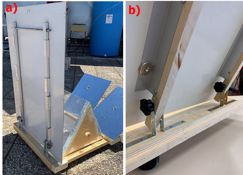
Figure 5.6: Detail of the connection of the reflector supports to the wooden base: a) primary reflectors and b) secondary reflectors.
