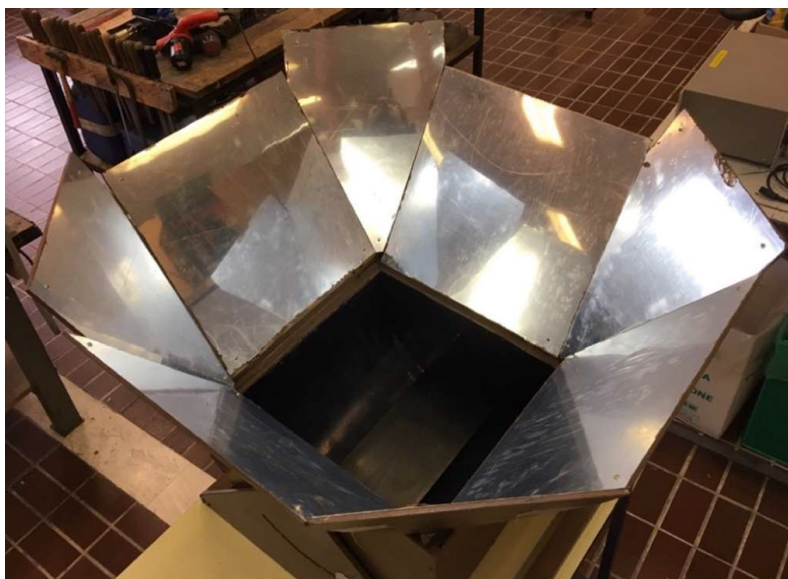
Figure 6.9: Final booster mirror system with a funnel-type shape.
