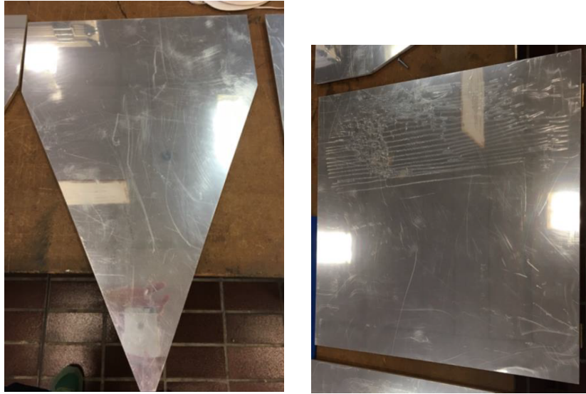
Figure 6.8: Square and wedge-shaped aluminum mirrors.
