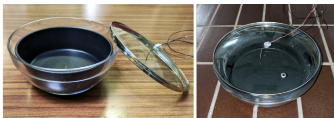
Figure 5.19: Receiver components (on the left); detail of immersed temperature sensor (on the right).
