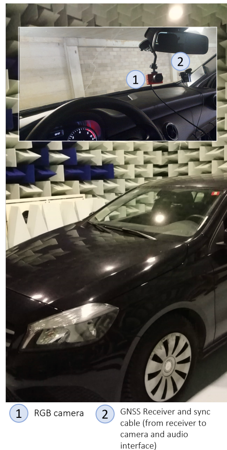
Fig. 3. Detail of the dashboard of the car equipped with the camera and the global navigation satellite system (GNSS) receiver.
